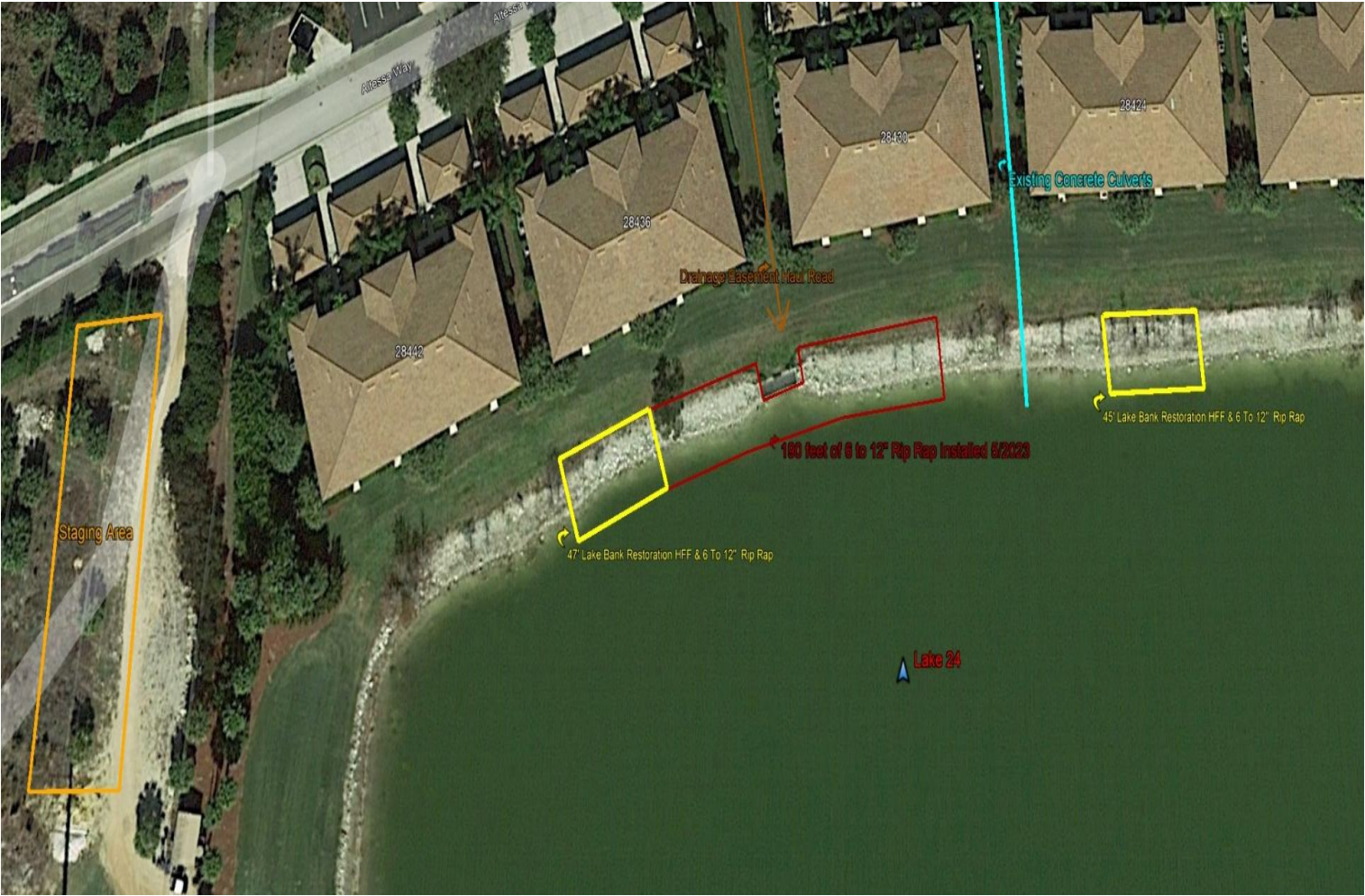
Exhibit: Staging & Work Areas for North 6 to 12" Rip Rap Installation on Lake 24.
