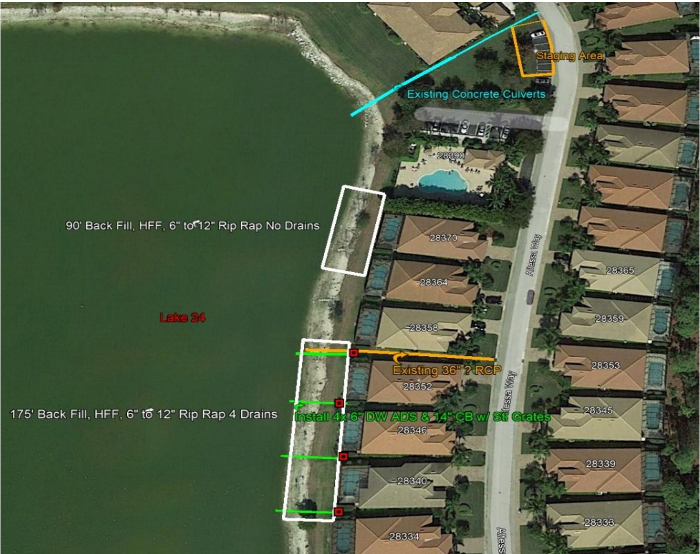
Exhibit: Staging & Work Areas for 6" Drainage & 6 to 12" Rip Rap Installation on Lake 24.
